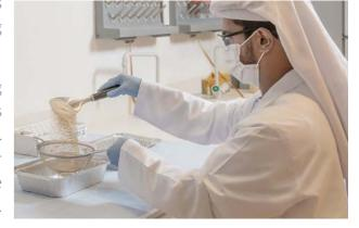
The Laboratory has samples preparation and analysis Standard Operating Procedures (SOPs) for non-destructive analysis using gamma spectrometry based on (HPGe) detector. All the collected samples prepared and analysed in the laboratory according to FANR laboratory's respective procedures.
